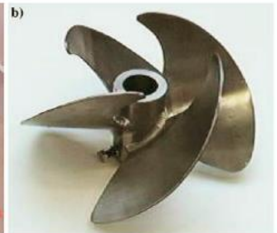
BME Fig. 13 (a) An ABEC 'elephant ear' impeller (used down-pumping); (b) Hayward Tyler up-pumping B2 hydrofoil
